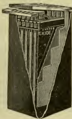
FIG. 431.—The Exide storage cell. The positive and negative plates are separated by thin sheets of perforated hard rubber, placed on both sides of each positive plate. The electrolyte and plates are contained in a hard rubber jar.
